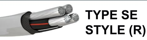
**APPLICATION:** KINGWIRE Service Entrance Cable Style R (SER) is used to convey power from the service drop to the meter base and from the meter base to the distribution panel board. It can be used for both above ground service entrance and interior wiring applications at temperatures not to exceed 90°C. The voltage rating is 600V.
